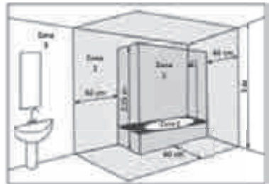
Zone 1: Appliances supplied to Safety Extra Low Voltage (SELV). Zone 2: Electrical Appliances Class II – IP X4 Zone 3: Electrical Appliances protected by RCD 30mA
